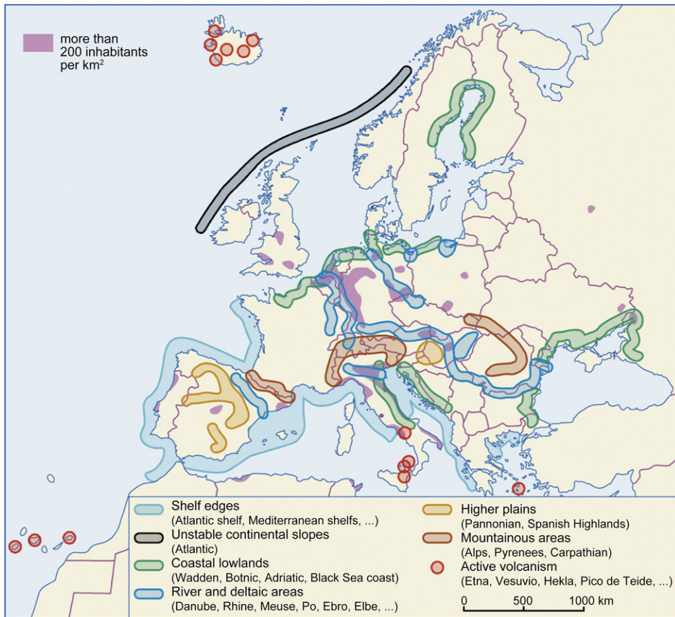
Fig. 1. Areas of vulnerability due to vertical movements in Europe, demonstrating the link between demography and environmental tectonics in Western and Central Europe (after Cloetingh et al., 2006b).
