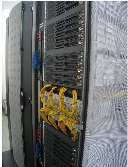
Fig. 14. Tectonic High Performance Simulator (Tethys) with 150 Processors, 150 Gbytes main memory and sustained performance for Earth System models in excess of 300 Gflops. This topical computing system is available to TOPO-EUROPE (courtesy H.P. Bunge).
